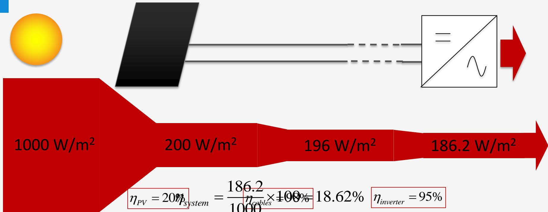
$$\eta_{system} = \eta_{PV} \times \eta_{cable} \times \eta_{inverter}$$
